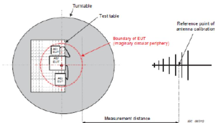
Figure C.1 – Measurement distance
